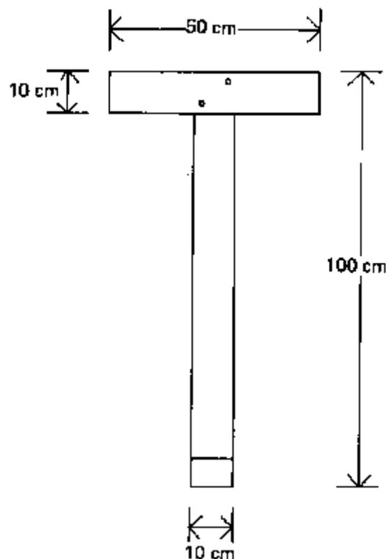
It is important that all boning rods have exactly the same height (100 cm) and while working with the boning rods, the sun should be kept in the back, as it would otherwise be difficult to see them. Usually a total of 3 or 4 boning rods is required.
