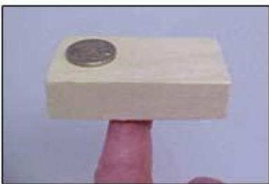
If the coin is moved toward one end of the block, the center of gravity moves toward that end, as well. This is because the weight distribution has changed. However, the block and off-center coin can still be supported by a finger pushing upward beneath the new center of gravity of the block-and-coin combination. Note the slightly off-center location of the supporting finger in the photograph below.
