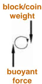
Once again, the center of buoyancy shifts to the left of center. The buoyant force acting upward through the center of buoyancy is the restoring force. When the downward push is removed, the restoring force tilts the block back to its original position.
