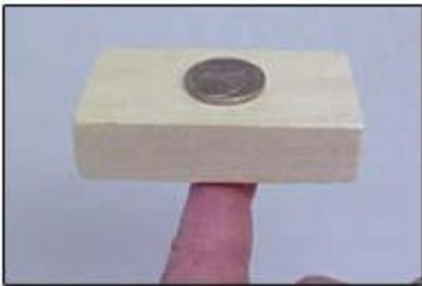
The position of the center of gravity of an object changes if there is a change in the distribution of weight. For example, if we place a coin on top of the wood block, the location of the center of gravity for the combination of the block and the coin is a little higher than for the block alone, because of the added weight of the coin. However, the block and coin can still be supported by a finger pushing upward beneath the center of gravity of the block-and-coin combination.
