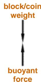
At this point, the upward buoyant force acting at the center of buoyancy exactly balances the downward force of the combined block-and-coin weight acting through the center of gravity.
